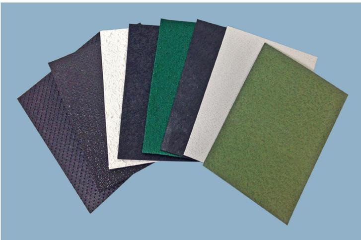
A coextruded textured geomembrane is controlled, to a great extent, by the addition of either a gas or a chemical that decomposes to a gas within the outer layers of a 3 or more layer coextruded geomembrane (Fig 1).
