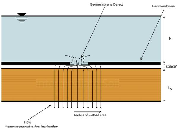
Figure 3 Composite liner variables
