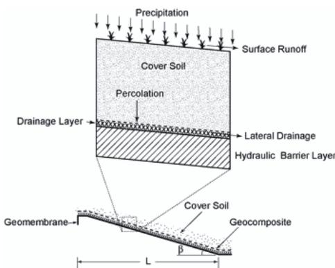
Figure 1 Disposition of precipitation in a typical final cover system
