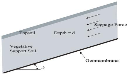
Figure 2 Seepage forces acting on side slope
