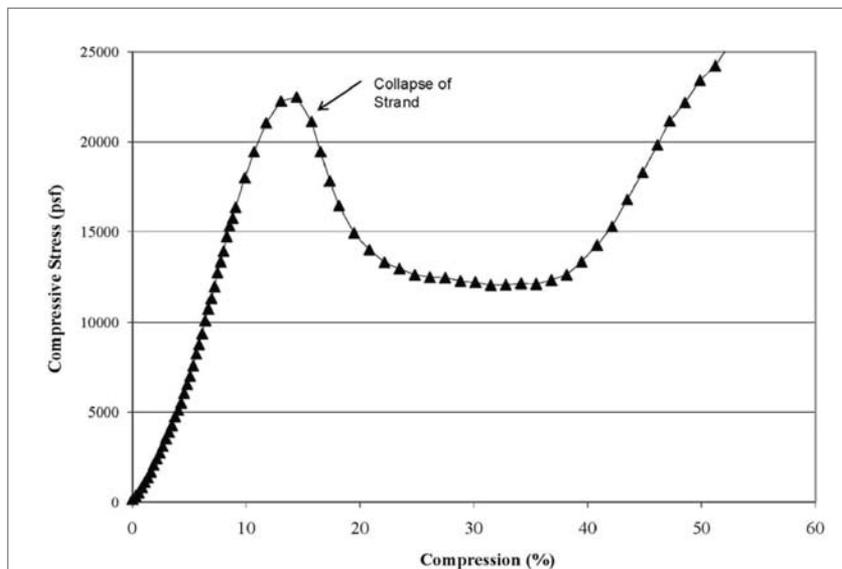
FIGURE 1 Compressive stress-strain behavior of biplanar geonets
