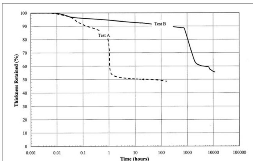
FIGURE 3 Creep failure in biplanar geonets
