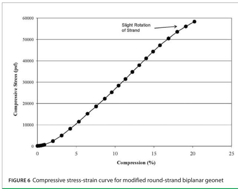
FIGURE 6 Compressive stress-strain curve for modified round-strand biplanar geonet
