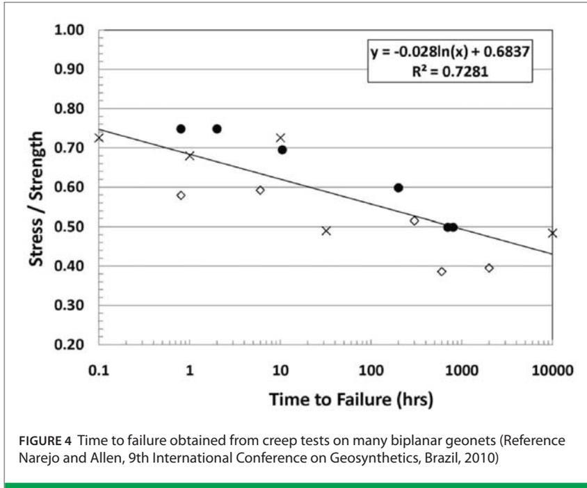
FIGURE 4 Time to failure obtained from creep tests on many biplanar geonets (Reference Narejo and Allen, 9th International Conference on Geosynthetics, Brazil, 2010)
