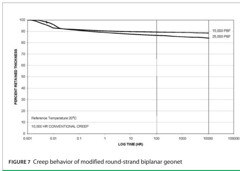
FIGURE 7 Creep behavior of modified round-strand biplanar geonet
