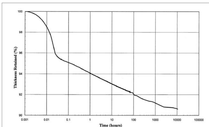
FIGURE 2 Example of a creep curve for a biplanar geonet
