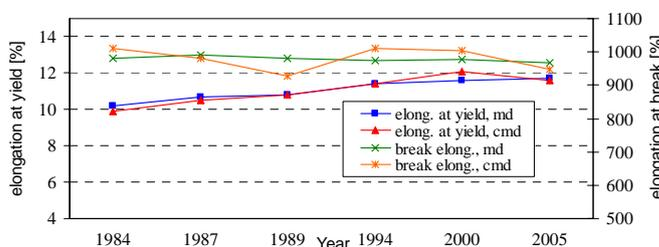
Figure 3. Galing II, change in elongation at yield and at break (acc. to ISO 527-3)
