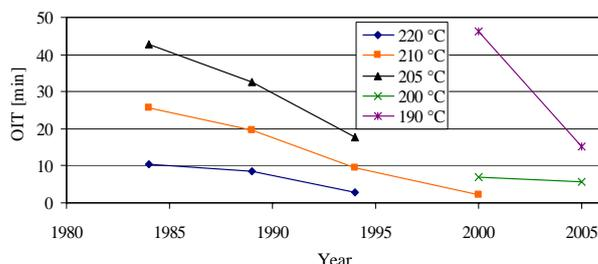
Figure 4. Galing II, OIT acc. to DIN EN 728 – Depletion of antioxidants
