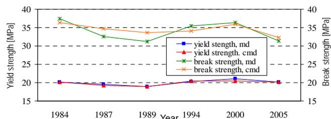
Figure 2. Galing II, change in tensile stress at yield and at break (acc. to ISO 527-3)
